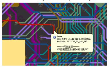
Because the circuit passes through the laser blind buried vias to all circuits, the blind buried vias of the circuit can be found after pressing F5. Light another end of the blind buried vias and judge the PCB layer where the circuit is located.
