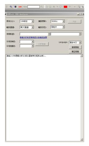
Using this software to analyze whether the communication of the bus external device on the corresponding model is normal, and the device bit number is used to judge whether the external device is damaged. Detailed usage functions are described in the instruction document for the logic analyzer.
